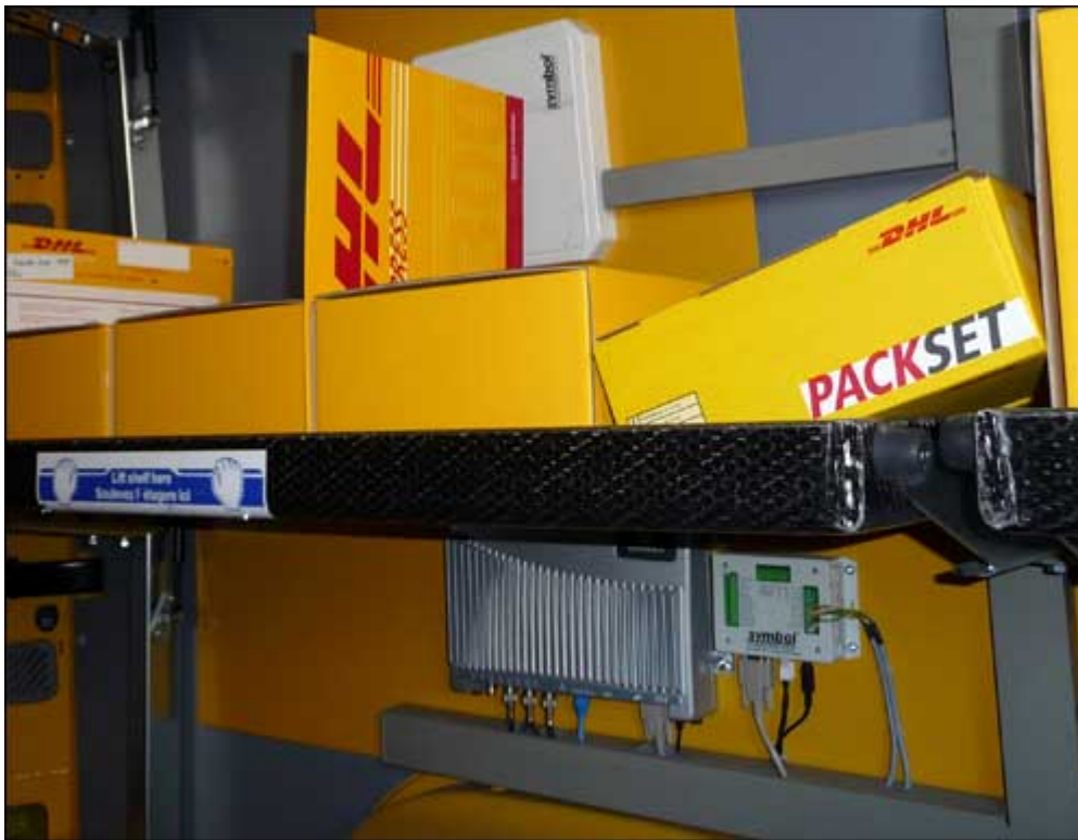
Each van has been outfitted with a Symbol (Motorola) XR 480 RFID interrogator connected to an onboard computer.
